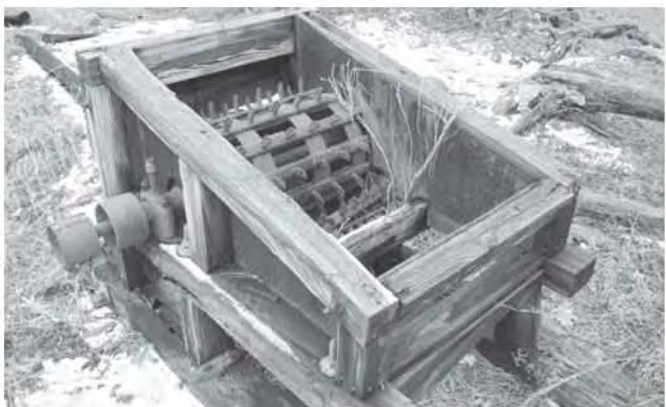
Figure 4. Late 19th century threshing machine with cast iron mechanism and teeth. Note similar shape of teeth to those found at Montpelier. ( http://dennisforney.files.wordpress.com )
